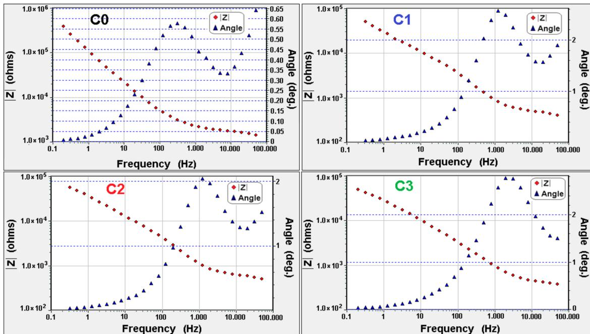
Figure 8. Bode diagrams for polymeric membranes with SiO<sub>2</sub> nanoparticles, before (C0) and after (C1–C3) 1 h of treatment.
