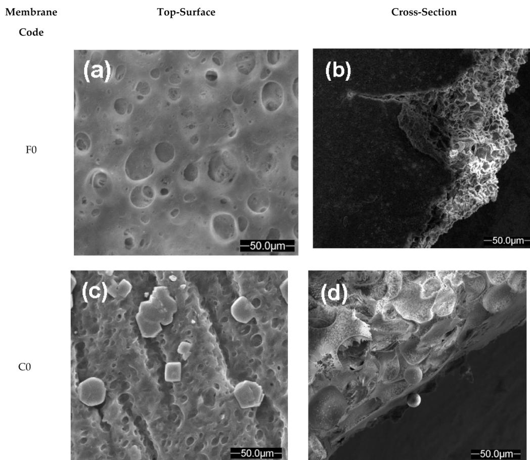
**Figure 6.** SEM images of polymeric membranes (without and with  $\text{SiO}_2$  nanoparticles): F0, top-surface (a) and cross-section (b); C0, top-surface (c) and cross-section (d).
