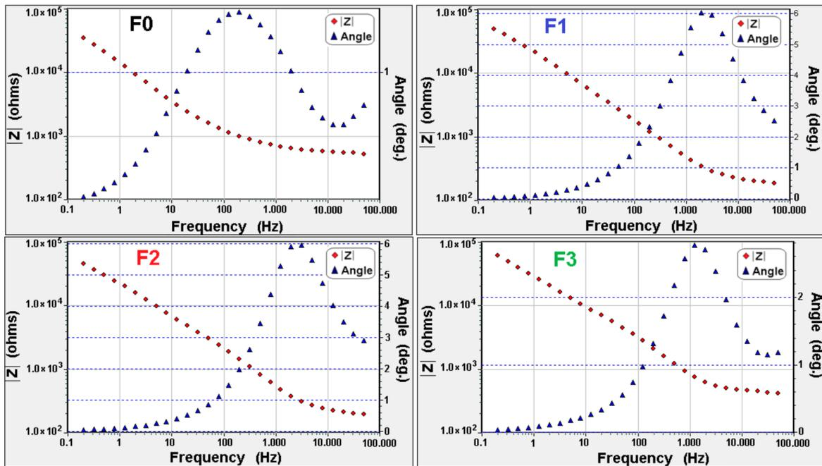
Figure 7. Bode diagrams for polymeric membranes without SiO<sub>2</sub> nanoparticles, before (F0) and after (F1–F3) 1 h of treatment.
