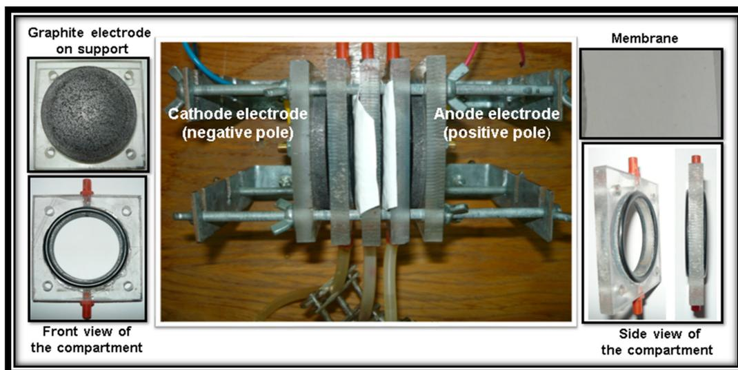
Figure 2. Laboratory electro dialysis system with polymeric membranes.
