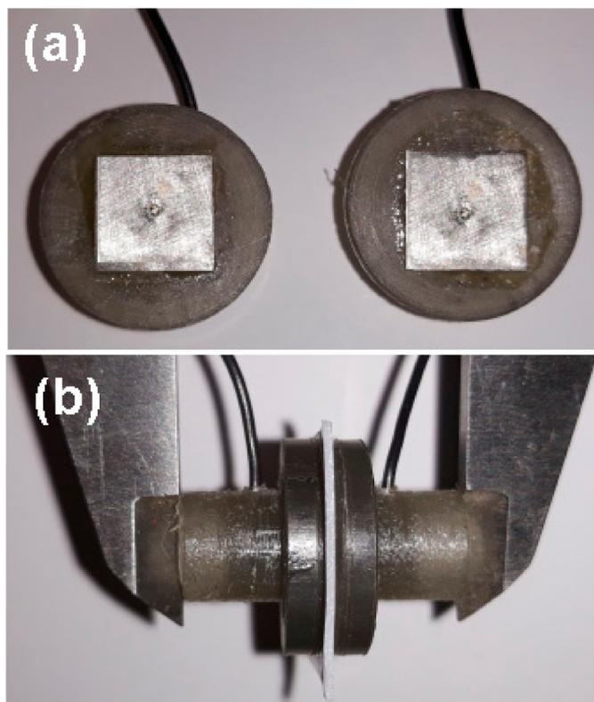
**Figure 3.** Electrochemical cell for EIS measurements: (a) two symmetrical platinum electrodes and (b) small sample of wet prepared polymeric membrane placed between platinum electrodes.
