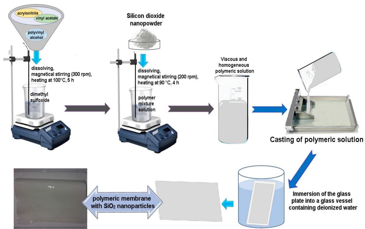
**Figure 1.** Schematic representation of the preparation polymeric membrane with SiO<sub>2</sub> nanoparticles.
