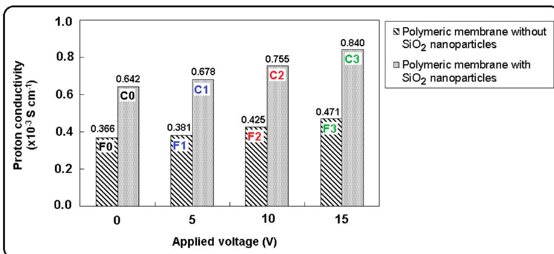
**Figure 9.** Proton conductivity values of polymeric membranes without and with SiO<sub>2</sub> nanoparticles, before and after used in the electro dialysis system.
