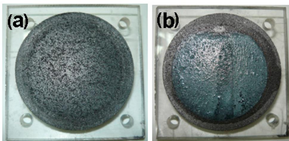
**Figure 4.** Image of cathode electrode surface before (a) and after (b) metallic zinc layer deposited.
