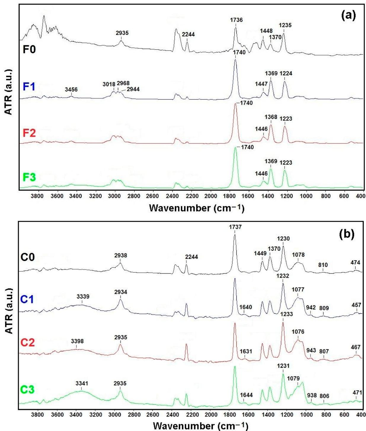
**Figure 5.** FTIR-ATR spectra for polymeric membranes without (a) and with (b) SiO<sub>2</sub> nanoparticles, before (F0 and C0) and after (F1–F3 and C1–C3) 1 h of treatment.
