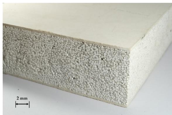
**Figure 4.** Example of Expandable Polystyrene Concrete Sandwich Wall.
