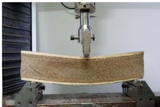
Figure 5. Three-point bending test of SIP prototype.
