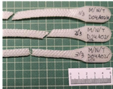
Figure 15. Triangular internal structure of M/N/T specimens.
