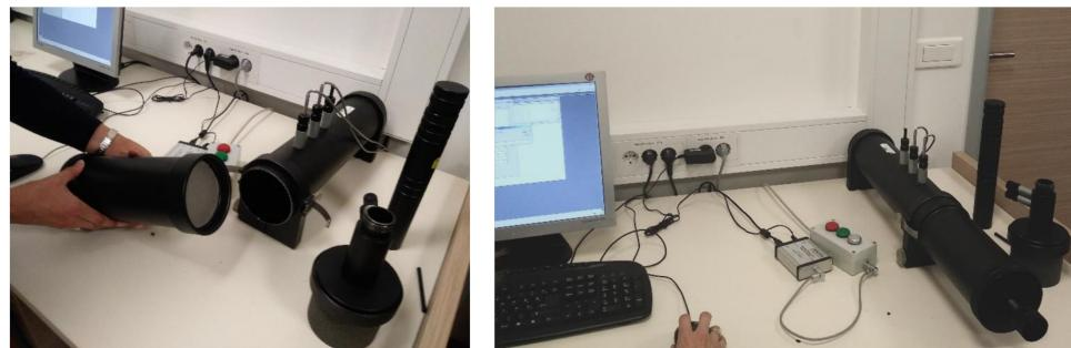
**Figure 6.** Open impedance tube with the inserted specimen (**left**) and assembled impedance tube ready to conduct the experiment (**right**).
