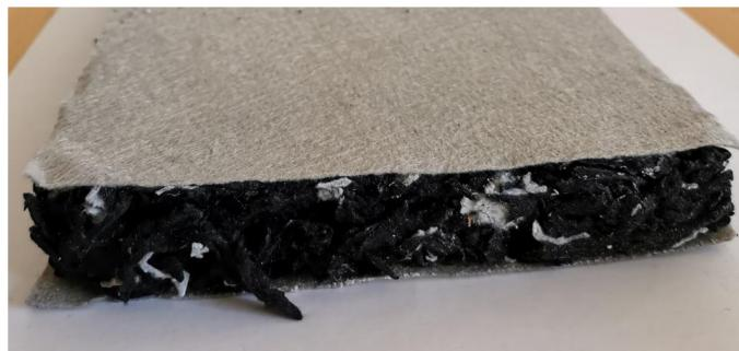
**Figure 2.** Thermal insulation slab made of shredded compressed waste polyester nonwoven textile.
