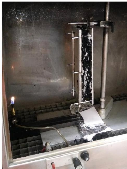
**Figure 5.** Reaction to fire test set-up for thermal insulation specimens according to the standard ISO 11925-2:2020 [38].
