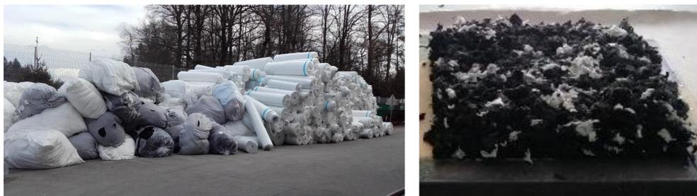
**Figure 1.** The discarded nonwoven polyester textile at the company's waste storage (left) and shredded waste polyester nonwoven textile prepared for further processing and manufacturing (right).
