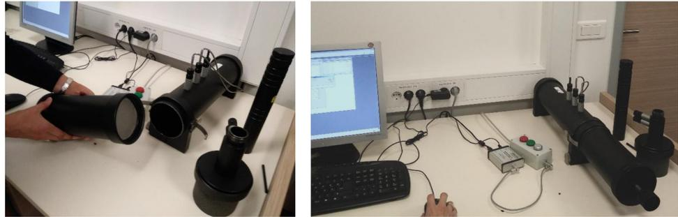
**Figure 6.** Open impedance tube with the inserted specimen (left) and assembled impedance tube ready to conduct the experiment (right).
