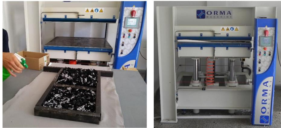
**Figure 3.** Applying of water glass on the shredded waste nonwoven textile (**left**) and pressing of the prepared material in the preheated hydraulic press (**right**).
