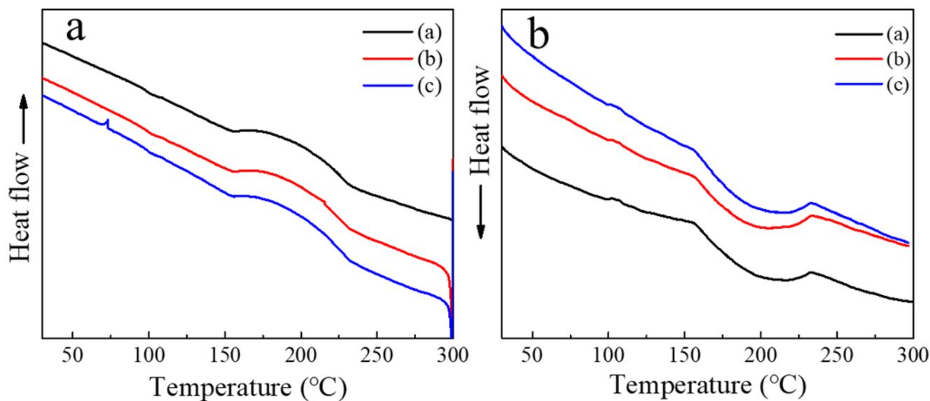
Figure S3 The DSC curve of cooling process(a) and heating process(b) ((a): ANF membrane, (b): ANF/HANF membrane, (c) HANF)
