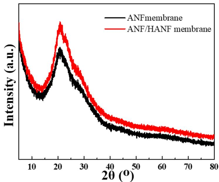
Figure S4 XRD patterns of the ANF membranes and ANF/HANF composite membranes (HANF: 50wt% of ANF)
