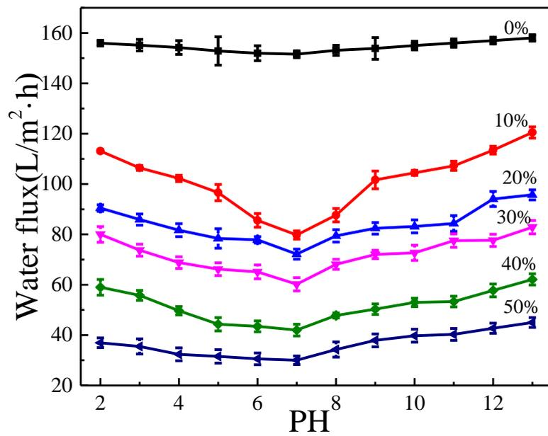
Figure S2 Trans-membrane fluxes of aqueous solutions at different pH values across ANF/HANF membranes with different contents of HANF
