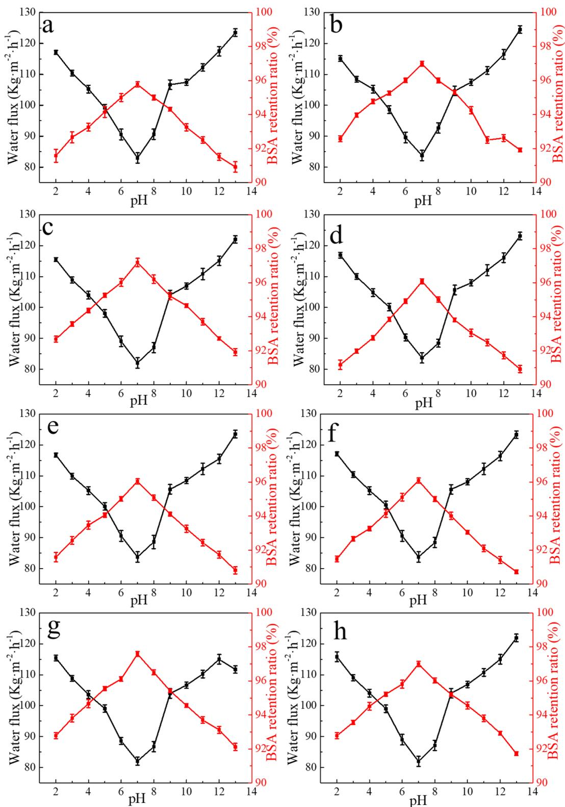
**Figure S5.** The variation of water flux (black line) and BSA retention ratio (red line) of the membranes after soaked in different solvent (a: DMSO; b: NMP, c: DMF, d: DMAC, e: THF, f: DMC, g: PhMe, h: MeOH) for 15 days with pH value.
