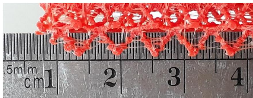
**Figure 10.** Multiple adjacent struts (lattice structure 1, ABS, Ender 3 scale 1.25:1). Nominal strut thickness 0.9 mm.
