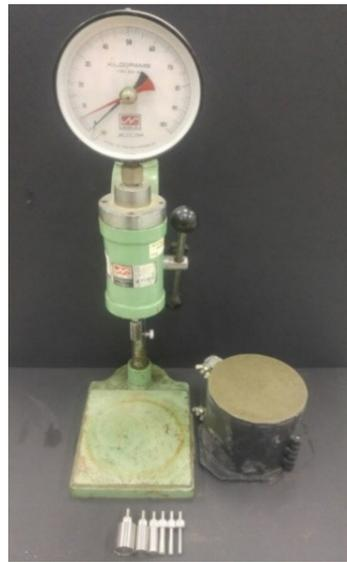
**Figure 3.** Test setup for set time measurement.
