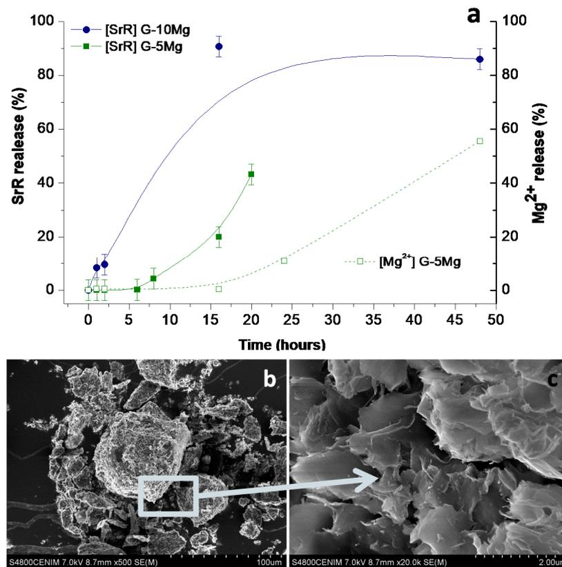
**Figure 4.** (a) Sr<sup>2+</sup> and Mg<sup>2+</sup> concentration determined by inductively coupled plasma (ICP) in the immersion medium during the degradation of G-5Mg and G-10Mg granules in phosphate buffer solution PBS and (b) Mg particle covered by polylactic acid (PLA) (c).
