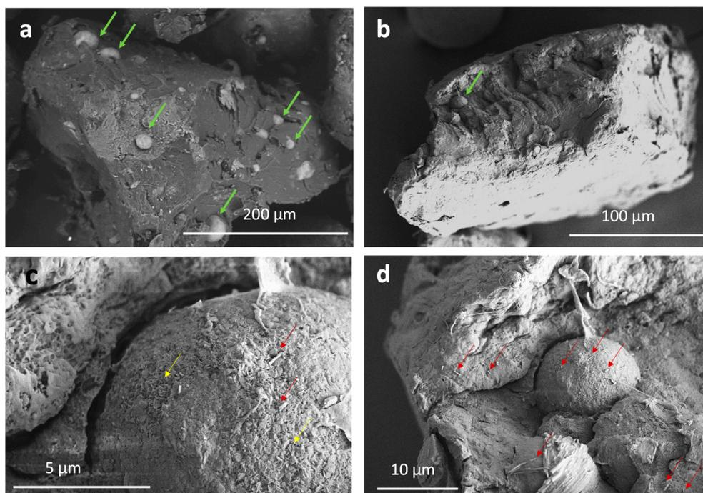
**Figure 3.** Micrographs of G-10Mg granules at different magnifications, highlighting (a,b) Mg particles (green arrows), (c,d) HNT-SrR (red arrows) and (c) the formation of MgO/Mg(OH)<sub>2</sub> nanoplatelets (yellow arrows).
