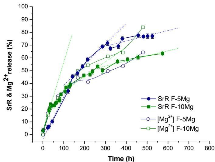
**Figure 7.** The cumulative release of SrR determined by UV–Vis spectroscopy and the  $Mg^{2+}$  concentration determined by ICP in the immersion medium during the degradation of F-5Mg and F-10Mg films in PBS.
