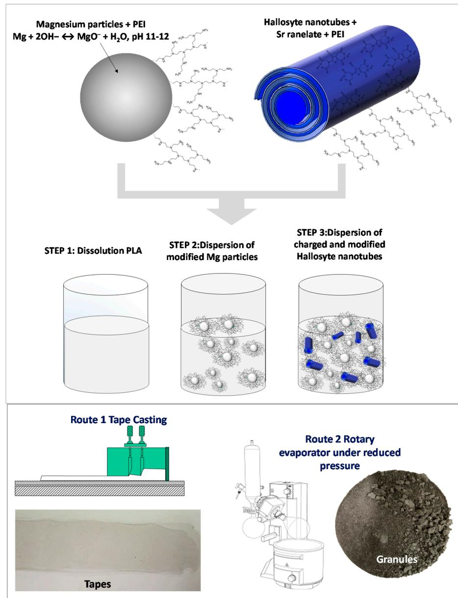
**Figure 1.** Scheme of the fabrication procedure of films and granules.
