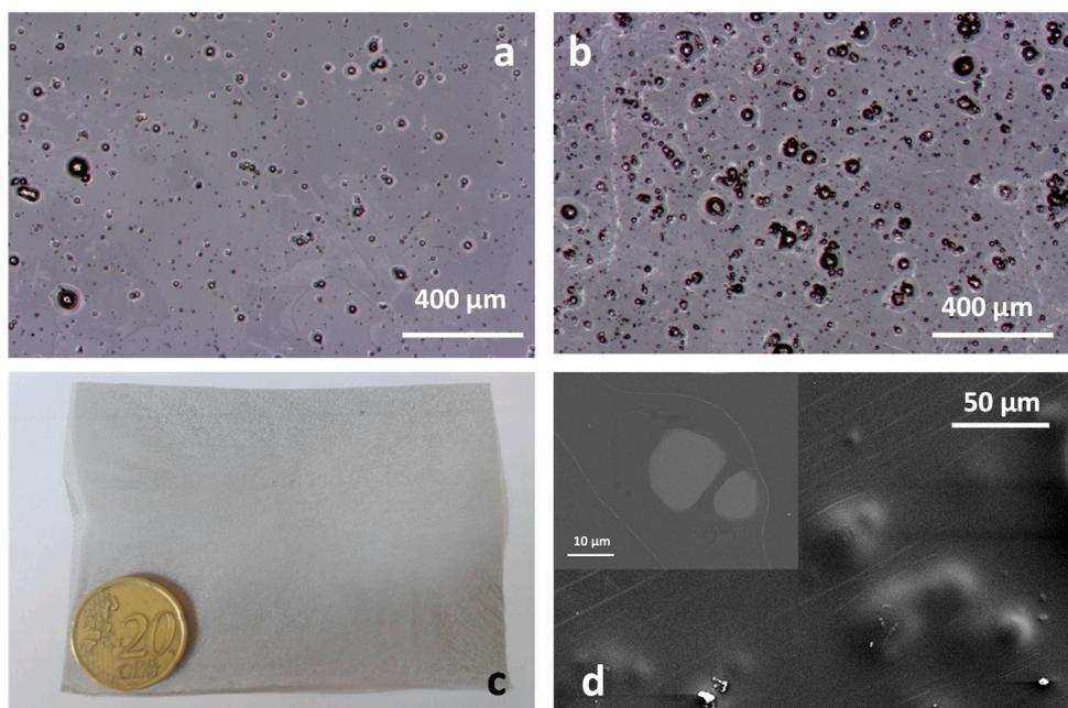
**Figure 6.** General view of the surface of F-5Mg (a) and F-10Mg (b) films, a macroscopic view of the film (c), and a detail of the surface of the imbibed Mg particles fully covered by the PLA (d).
