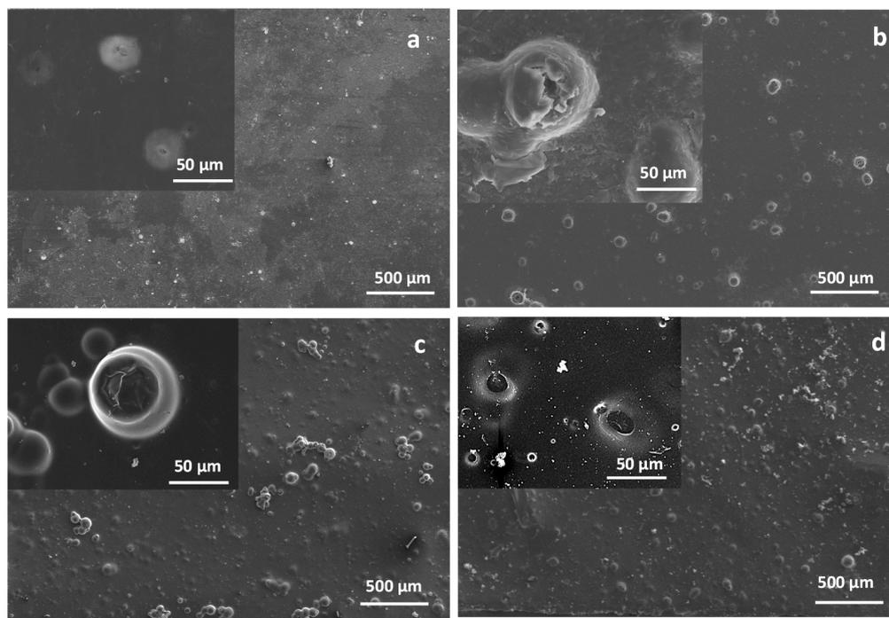
**Figure 8.** General view of the surface of F-5Mg films degraded for 100 h (a) and 265 h (b), and of F-10Mg films degraded for 170 h (c) and 500 h (d). At the insets, a detail of the degradation of Mg particles and surrounding PLA matrix is shown.
