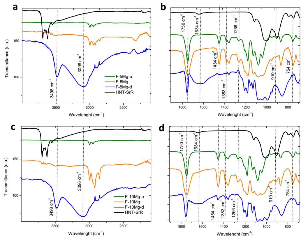
**Figure 9.** Depicts the complete FTIR spectra of F-5Mg-u, F-5Mg, and F-5Mg-d (a,b) composites and F-10Mg-u, F-10Mg, and F-10Mg-d (c,d) films.
