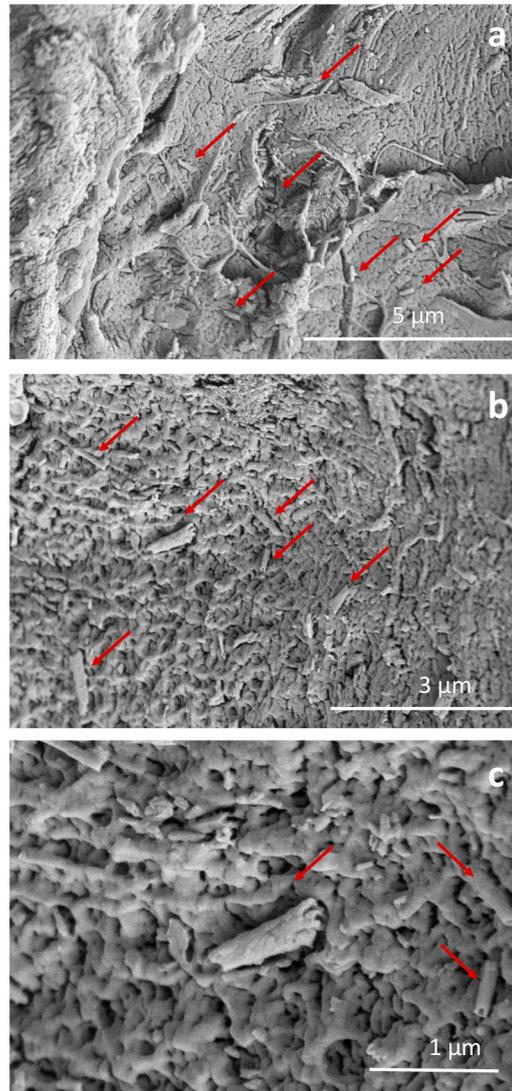
**Figure 2.** Micrographs of G-HNT granules at different magnifications, highlighting the dispersion of halloysite nanotubes–strontium ranelate (HNT–SrR) (red arrows) (a,b) and the nanotube morphology (c).
