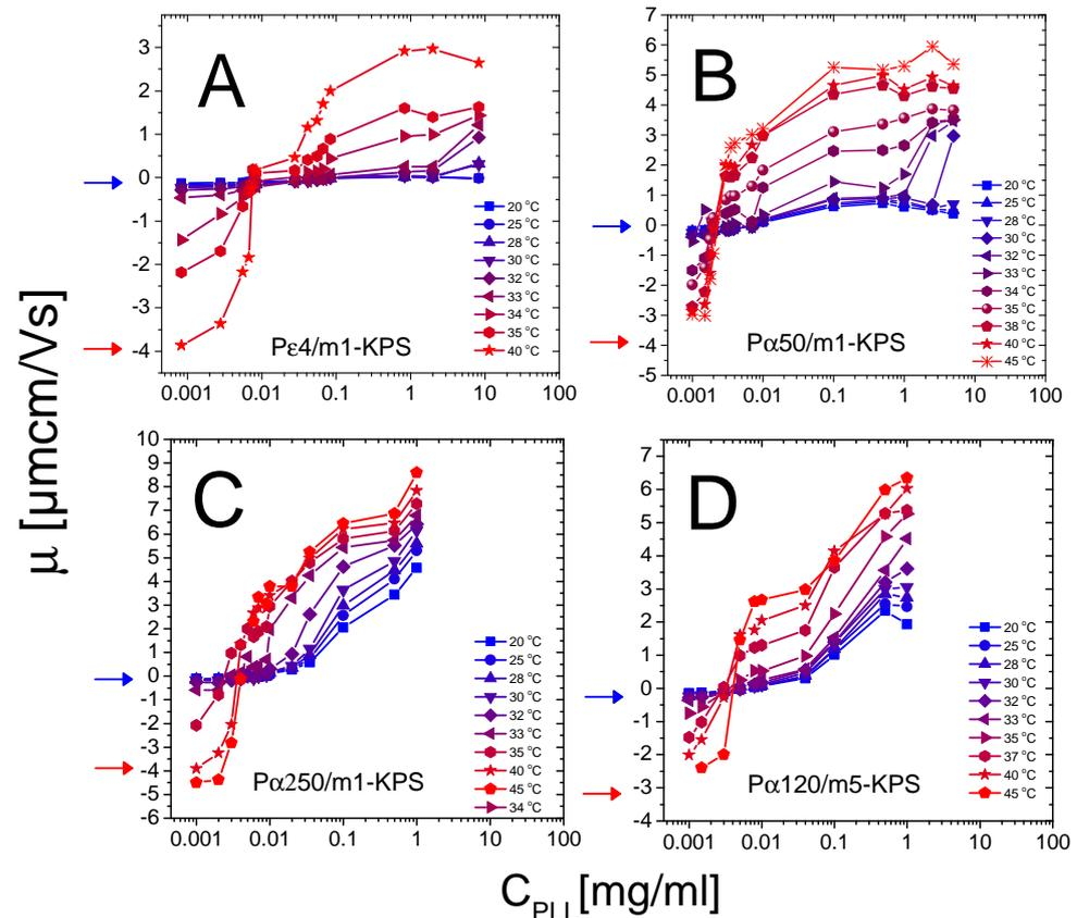
**Figure 5.** Electrophoretic mobility in function of  $C_{PLL}$  for  $P\epsilon 4/m1$ -KPS (Panel A),  $P\alpha 50/m1$ -KPS (Panel B),  $P\alpha 250/m1$ -KPS (Panel C) and  $P\alpha 120/m5$ -KPS (Panel D) mixtures, and selected temperatures as indicated in the panels. Mobilities of bare microgels at 20 °C (blue arrows) and 40 °C (red arrows) are also shown for reference.
