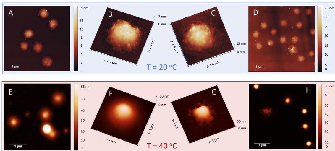
**Figure 10.** AFM images of  $P\alpha 250/m1$ -KPS complexes formed at  $C = 0.0015$  mg/mL (panels A,B and E,F) and  $C = 0.01$  mg/mL (panels C,D and G,H), for  $T < T_c$  (upper panel) and  $T > T_c$  (lower panel). The presence of the PLL shell surrounding microgels is particularly evident above  $T_c$  where a diffuse or globular-like corona is observed depending on PLL amount.
