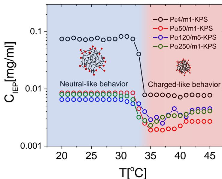
**Figure 6.**  $C_{IEP}$  in function of temperature for all the investigated PLL-microgel mixtures. The sudden drop of  $C_{IEP}$  in proximity of  $T_c$  marks the electrokinetic transition between the neutral-like and the charged-like state of PNIPAm microgels.
