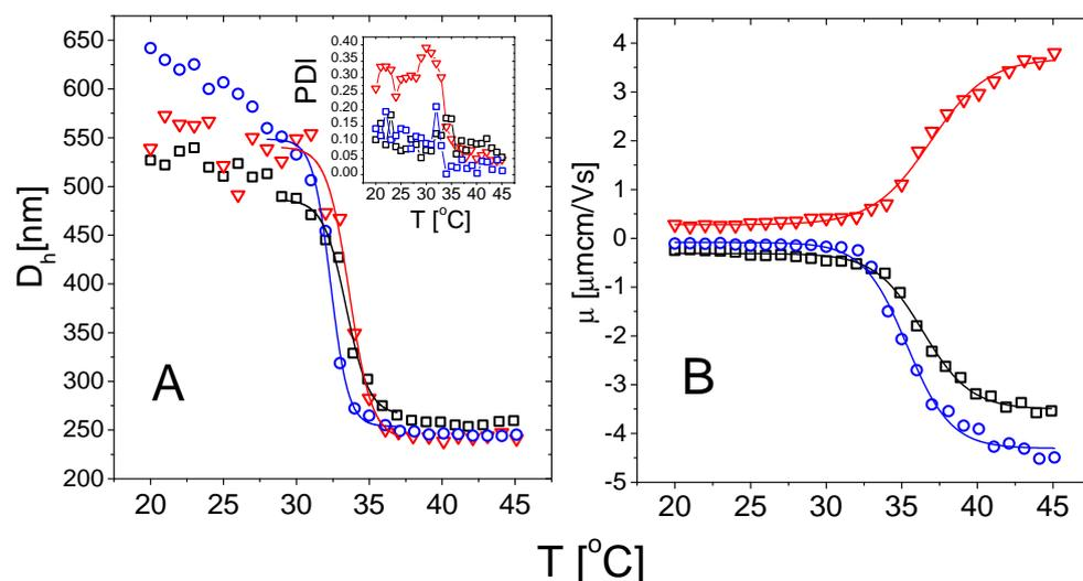
**Figure 3.** Hydrodynamic diameter (Panel A) and electrophoretic mobility (Panel B) of m1-KPS (circles), m5-KPS (squares) and m5-AIBA (triangles) microgels in water as a function of temperature. Solid lines are fits obtained using Boltzmann functions as detailed in the text. The inset (Panel A) shows the polydispersity index (PDI) obtained via a cumulant analysis of the intensity autocorrelation functions  $g_2(\tau) - 1$  for the three microgel types.
