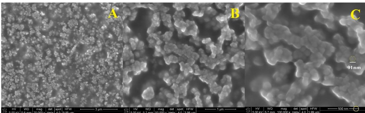
**Figure 8.** SEM images of nanospheres suspension 3 enlarged 20,000 times (A), 50,000 times (B) and 100,000 times (C).
