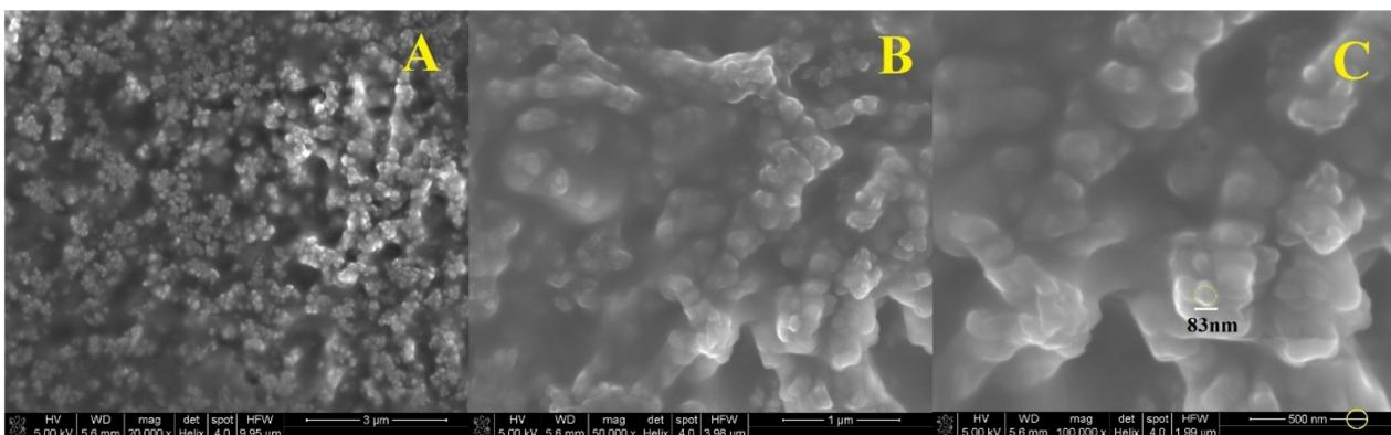
**Figure 7.** SEM images of nanospheres suspension 2 enlarged 20,000 times (A), 50,000 times (B) and 100,000 times (C).
