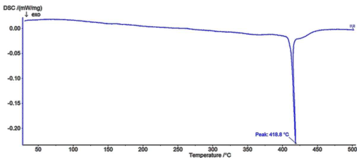
Figure 11. DSC spectra of PHMW DSC spectra of high molecular weight polymer.
