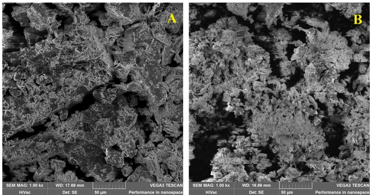
Figure 4. SEM images of (A) the  $\beta$ CD (1000 $\times$  zoom) (B) the Pa $\beta$ CD (1000 $\times$  zoom).
