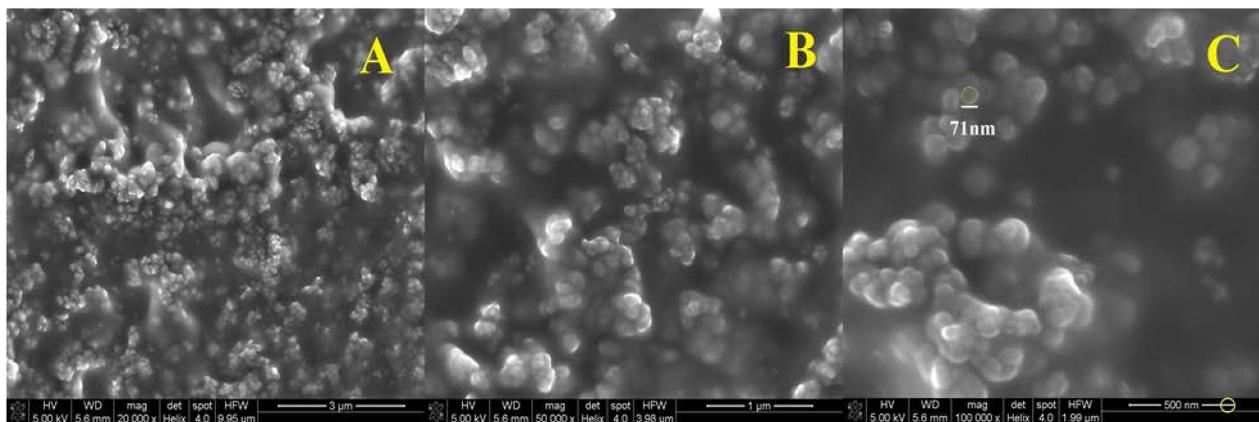
**Figure 6.** SEM images of nanospheres suspension 1 enlarged 20,000 times (A), 50,000 times (B) and 100,000 times (C).
