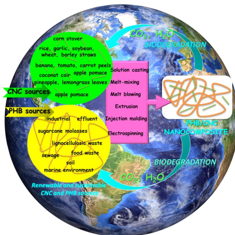
**Figure 1.** Circuit of biodegradable PHB/CNCs nanocomposites in the context of a circular economy.
