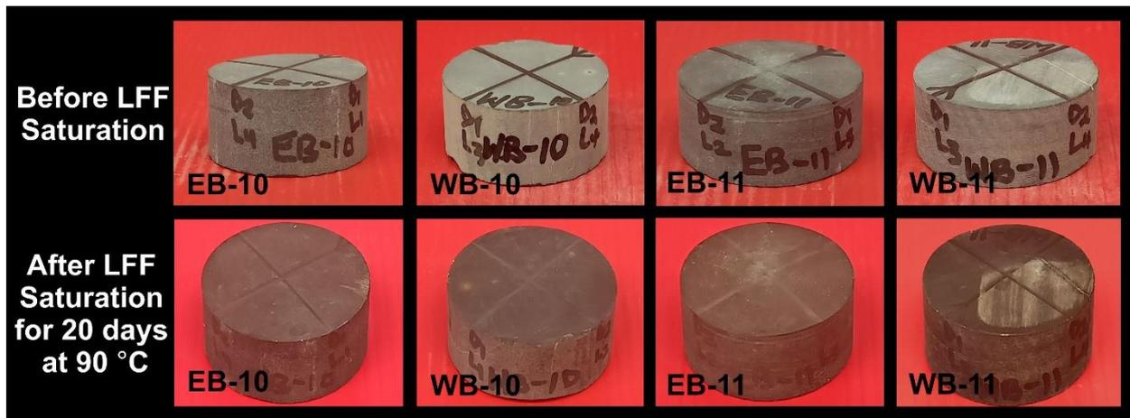
Figure 11. Pre- and Post-LFF saturations of Eagle Ford and Wolfcamp shales at 90 °C for a period of 20 days. EB-10 and WB-10 were LFF<sub>1</sub> saturated, while EB-11 and WB-11 were LFF<sub>2</sub> saturated.
