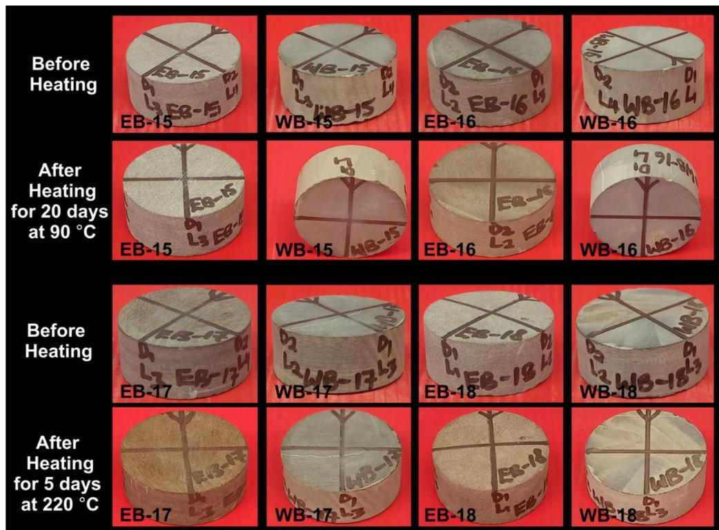
Figure 12. Pre- and Post-thermal conditioning of Eagle Ford and Wolfcamp shales for the periods of 20 days at 90 °C for EB-15, EB-16, WB-15, and WB-16 and 5 days at 220 °C for EB-17, EB-18, WB-17, and WB-18.
