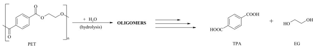
**Figure 5.** Neutral hydrolysis of PET [40].
