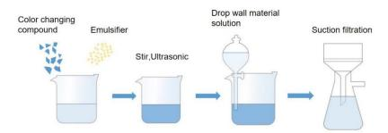
Figure 1. Microcapsule preparation process flowchart.
