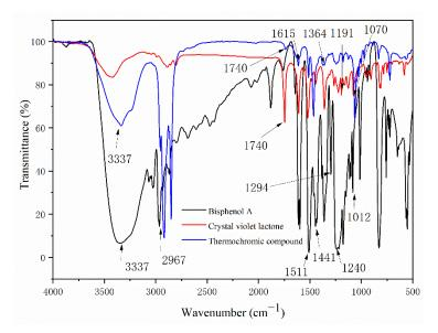
Figure 3. FTIR spectra of BPA, CVL, and the thermochromic compound.
