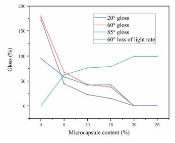
Figure 6. A gloss of coating with different microcapsule content.
