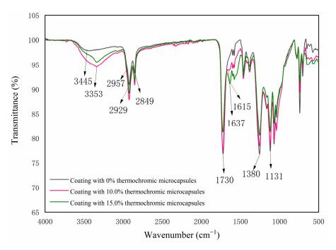
Figure 8. FTIR spectra of coatings with different microcapsule contents.
