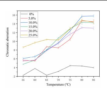
Figure 4. Effect of microcapsule content on the thermochromic difference of coating.
