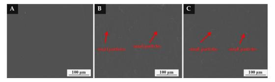
**Figure 7.** Morphology of coating with different content of microcapsules: (**A**) 0%, (**B**) 10.0%, (**C**) 15.0%.
