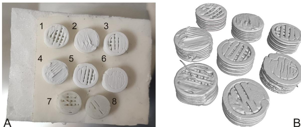
**Figure 3.** Samples for CT scanning: (A) sample storage (1—HS por; 2—HS solid; 3—PBS por; 4—PBS solid; 5—SS por; 6—SS solid; 7—non-degraded porous sample; 8—non-degraded solid sample); (B) visualisation of surface reconstruction of individual samples.
