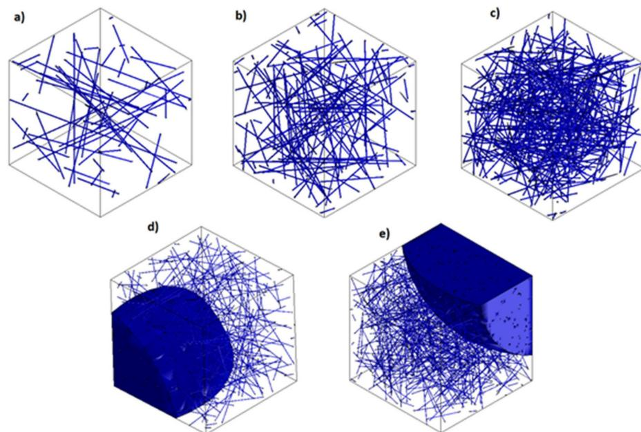
**Figure 1.** Generation of RVEs as a function of the percentage of nanofillers. (a) 0.5 wt.%; (b) 1 wt.%; (c) 2 wt.%; (d) 4 wt.%; (e) 5 wt.%.
