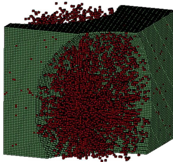
**Figure 7.** Aggregates/agglomeration of CNT in RVE matrix.
