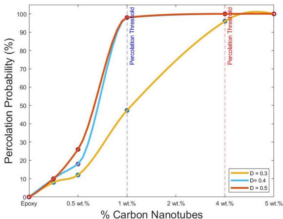
Figure 11. Percolation probability with different tunnelling distances.
