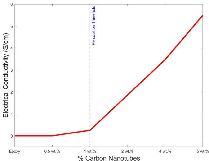
**Figure 10.** Experimental samples' electrical conductivity.
