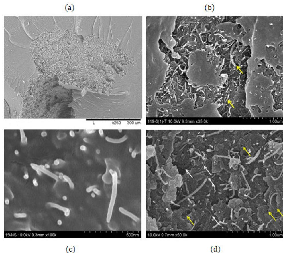
**Figure 5.** SEM characterization sample CNT 4%wt: (a) CNTs agglomeration, (b) high magnification of CNT agglomeration, (c) interface adhesion CNT and epoxy resin, and (d) CNTs and porosity characterization, Yellow arrows represent the Porosity, White allow point the CNTs.
