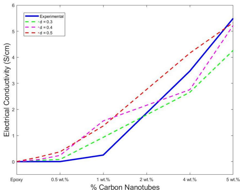
**Figure 12.** Comparison of electrical conductivity of MATLAB simulations with experimental data.
