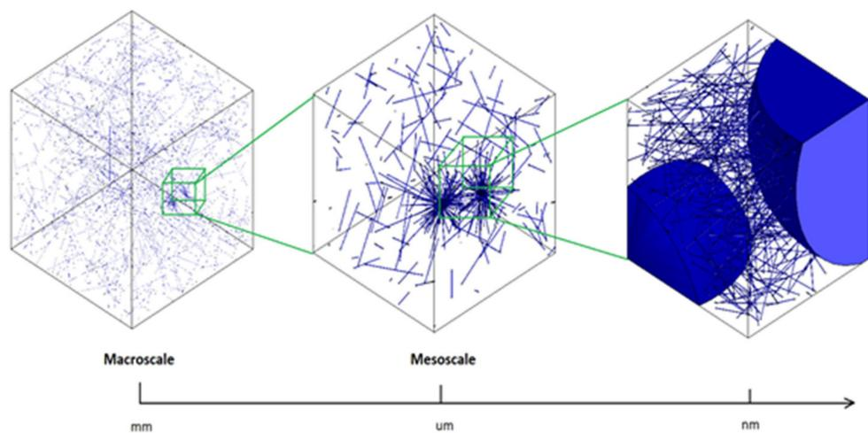
**Figure 2.** Schematic multiscale modelling of CNT agglomerations.
