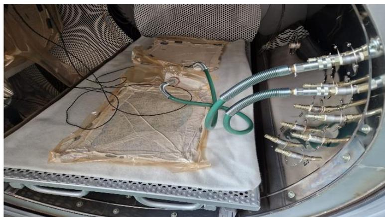
**Figure 1.** Autoclave curing procedure of GFRP samples.
