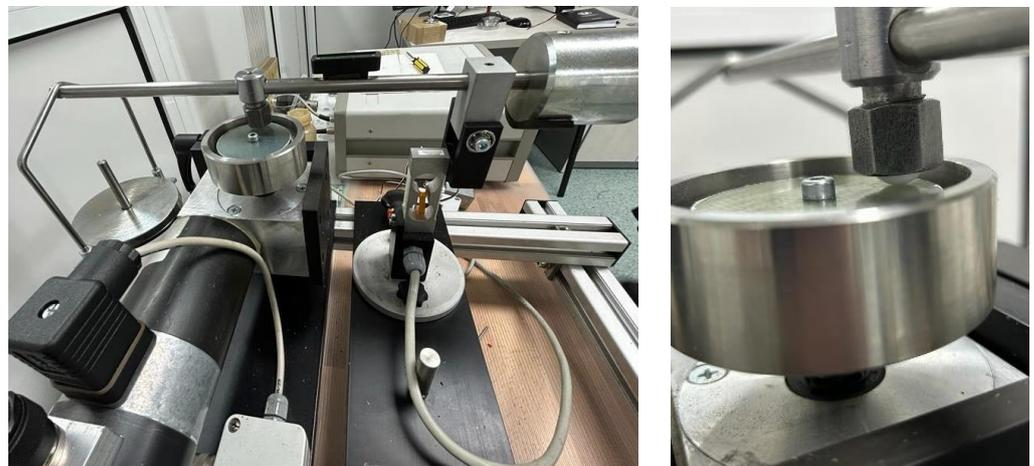
**Figure 7.** A modified pin-on-disc tribometer.
