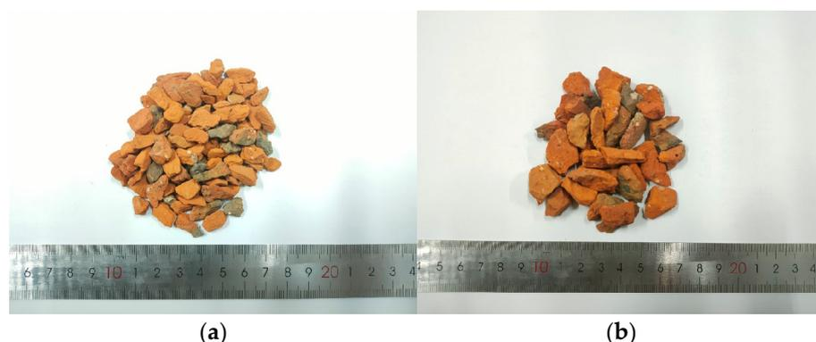
**Figure 2.** Recycled-brick aggregates: (a) Particle sizes ranging from 5 to 10 mm; (b) Particle sizes ranging from 10 to 20 mm.
