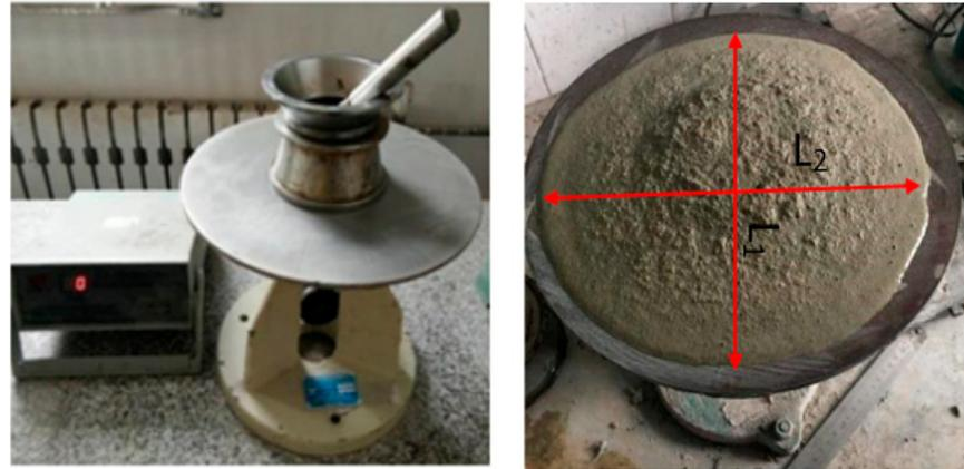
**Figure 7.** Slump flow test setup.
