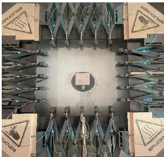
Figure 1. Diagram of the biaxially-oriented stretching process of BOPA-56/512.
