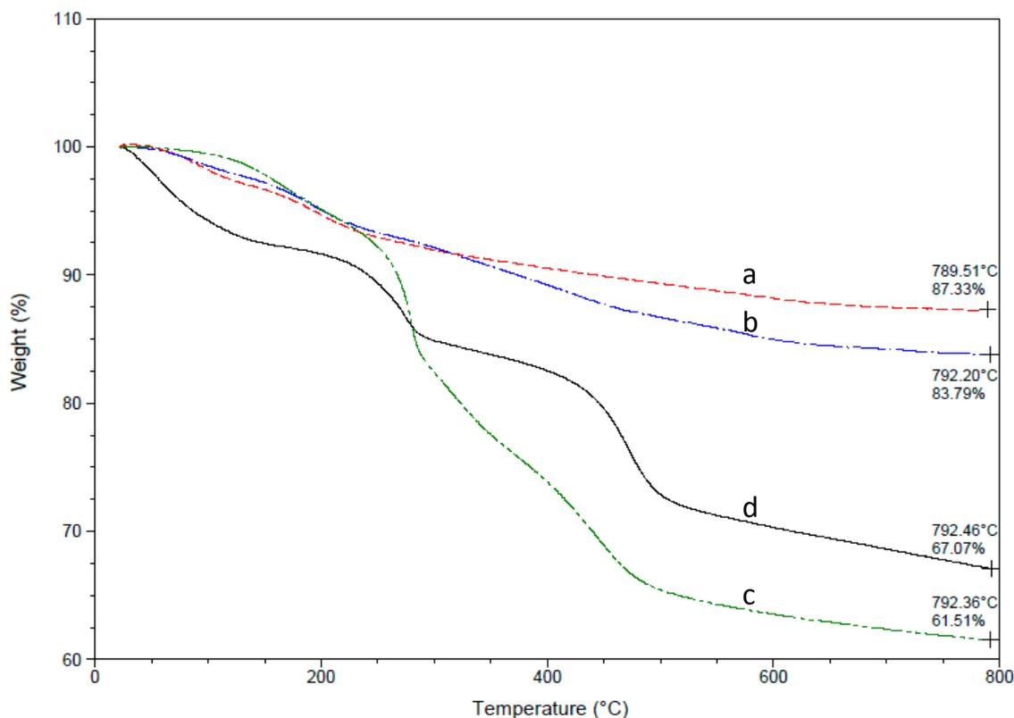
**Figure 1.** Thermo-gravimetric analysis (TGA) results of silica nano-particles (Si-NP) (diameter 200 nm) at various stages of decoration: (a) bare Si-NP; (b) initiator decorated Si-NP; (c) brush poly(*t*-BMA) decorated Si-NP (polymerization time 180 min.); (d) brush poly(methacrylic acid) (PMAA) decorated Si-NP. Note that all samples have been processed under the same conditions (freeze/drying for 5 days at 0.1 mPa at room temperature).
