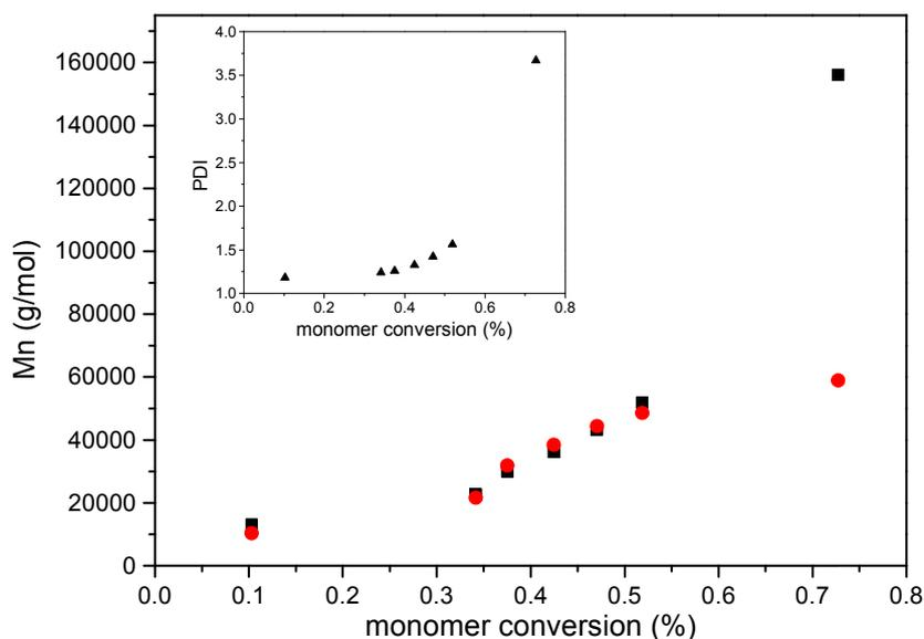
**Figure 3.** Molecular weights ( $M_n$ ) and polydispersity (PDI, inset,  $\blacktriangle$ ) of de-grafted polymer ( $\blacksquare$ ) and free polymer ( $\bullet$ ) as a function of monomer conversion.
