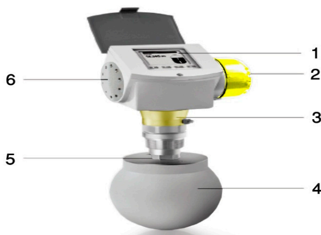
Figure 7. The catalyst dosing measurement device. (1) An elective touchscreen with a dose-controlling optional button; (2) A dual-wire reading meter; (3) A changeable and a rotatable converter consisting of a rapid connector technique; (4) Horn antennas (made of stainless steel); (5) A flange plate protector (needed for aggregating products) with extension services; (6) A single converter for many applications.
