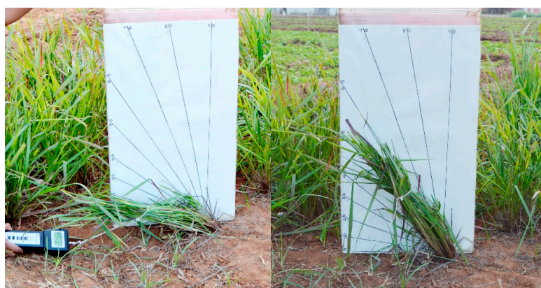
Figure 2. Push-pull gauge used to measure the culm strength in the mutant population.
