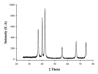
Figure 1. X-ray diffraction of the synthetic zinc oxide nanoparticle (Zincite-ZnO NP).
