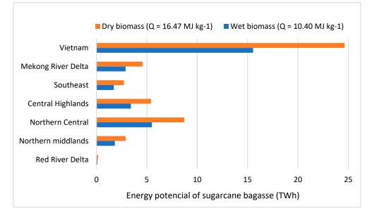
Figure 4. Impact of pretreatment on bagasse yearly energy potential.
