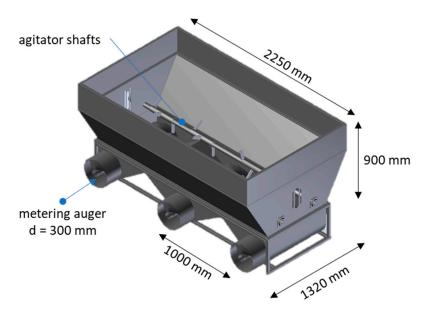
Figure 6. Compost tank with two hydraulically driven mixing and three metering augers.
