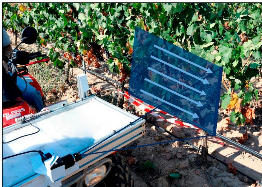
**Figure 1.** Hyperspectral imaging acquired on-the-go with a push-broom camera mounted on an all-terrain vehicle (ATV) at 5 km/h.
