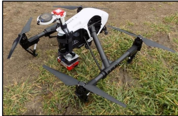
**Figure 2.** DJI Inspire 1 with a hitched Red Edge M camera. GPS receiver and the downwelling light sensor were mounted by using an ad hoc structure.
