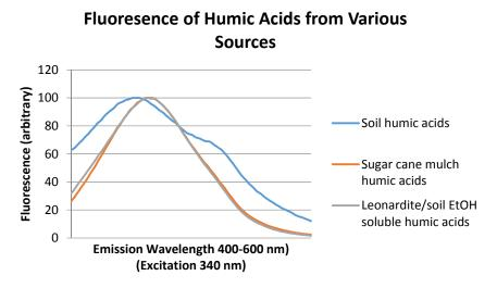
**Figure 2.** Fluorescence spectra of humic acids extracted from soil, sugar cane mulch, and Leonardite coal (NZ) (Leonardite/soil ethanol-soluble extracts were identical, so only one trace is shown).
