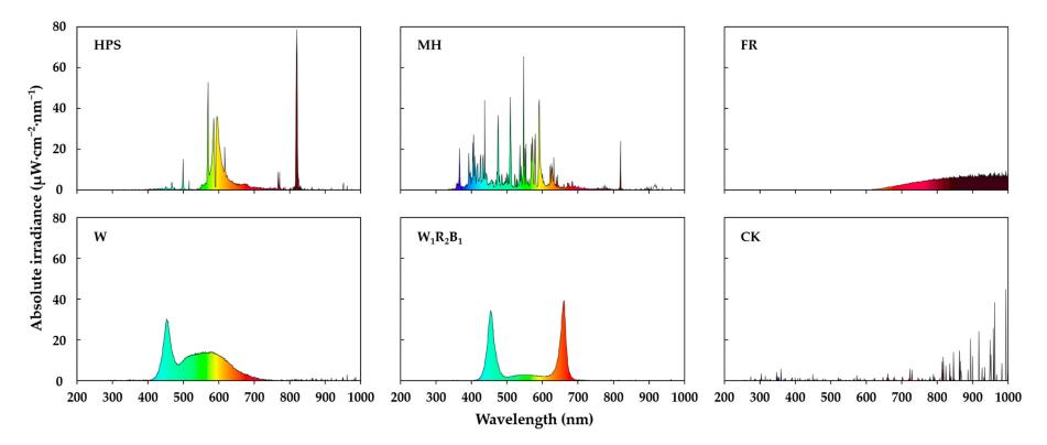
**Figure 2.** Spectral qualities of the different supplementary light sources used in the experiment. HPS (high-pressure sodium), MH (metal halide), FR (far-red), W (white LEDs), W<sub>1</sub>R<sub>2</sub>B<sub>1</sub> (mixed LEDs), and CK (control).
