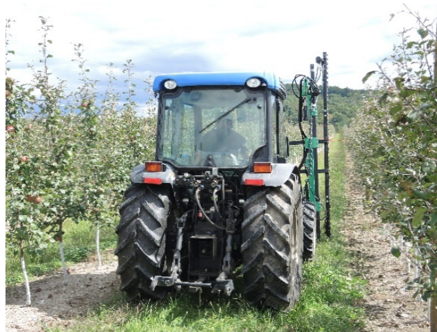
Figure 7. Mechanical pruning systems for apple trees with saw-tooth cutter driven by a tractor.
