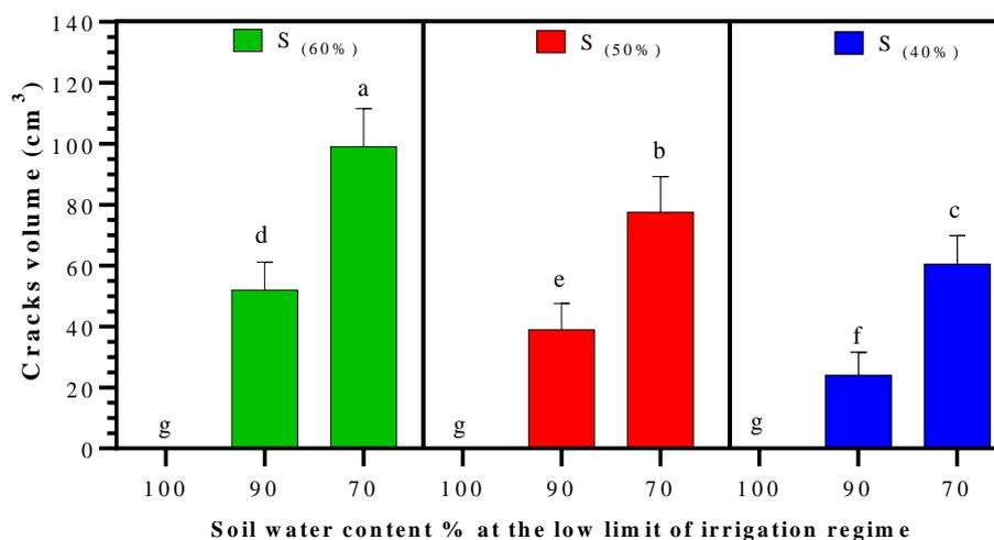
**Figure 2.** The crack volume due to soil water content and soil clay content in 2017. Values are means  $\pm$  SD. S (40%), S (50%), S (60%), representing soil clay contents of 40%, 50%, and 60%, respectively. The means are not significantly different when followed by the same letter.
