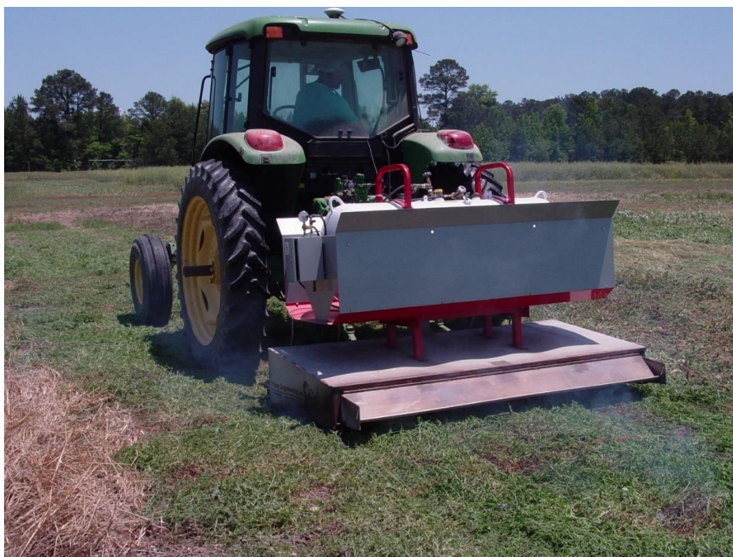
Figure 1. Rolled/cripped hairy vetch winter cover crop being desiccated by a Red Dragon® Flamer PL-8750 Poultry House Flame Sanitizer, Flame Engineering, Inc., moving at 1.2 k/h and emitting 1100 °C.
