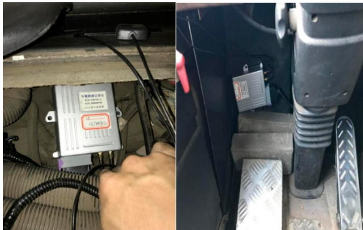
**Figure 1.** Vehicle engine data logger.
