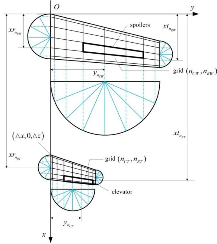
**Figure S1.** Grid distribution on wing and horizontal tail.
