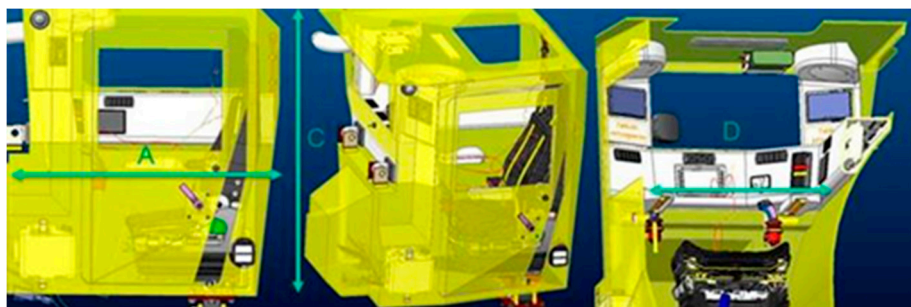
Figure 1. Cabin of a loader—autonomous mobile machine operating in underground mines. Internal dimensions: A—1275 mm, C—1335 mm, D—800 mm.
