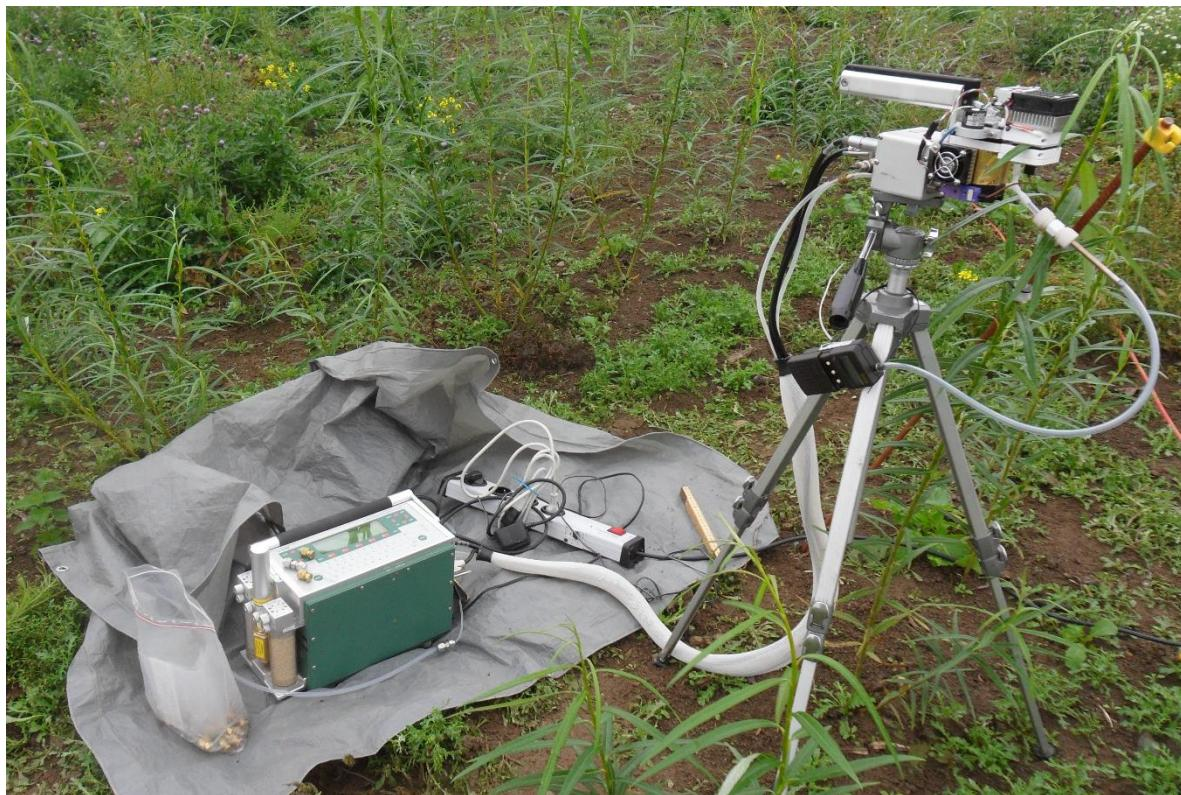
**Figure S1.** Experimental setup of leaf chamber system. To the right on the top of the tripod, the leaf chamber is attached and connected to the portable photosynthesis system (LI-6400) to the left. BVOC-sampling was done by taking a sub-sample of 200 ml/min of air leaving the leaf chamber using adsorbent tubes filled with Tenax TA and Carbograph with a small flow regulated pump.
