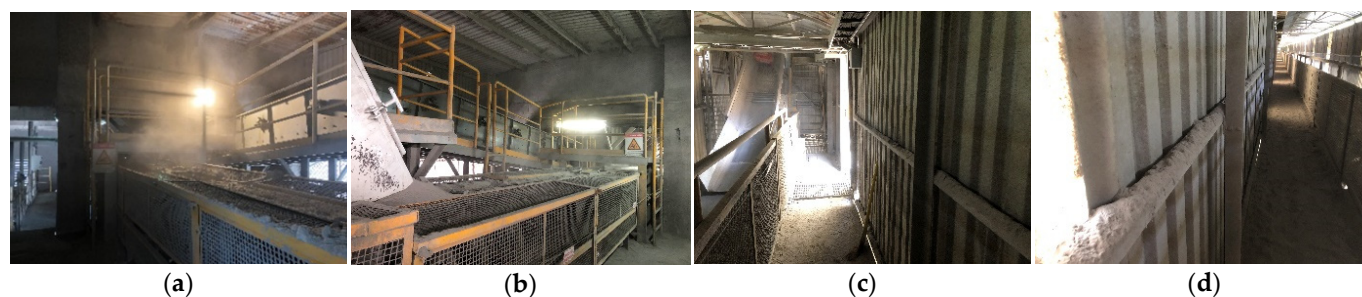
Figure 2. Some dust sources in the cement grinding plant: (a) mill inlet; (b) underneath of feed-bin; (c) at changed-direction point; (d) accumulated dust along dispatch belt conveyor.
