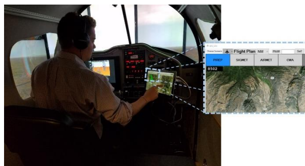
Figure 3. Weather and map display tablet in the cockpit. The arrival of a new weather message is indicated by the associated soft button highlighting in blue. Touching the soft button would open/close a pop-up text window that included the full text of the message.
