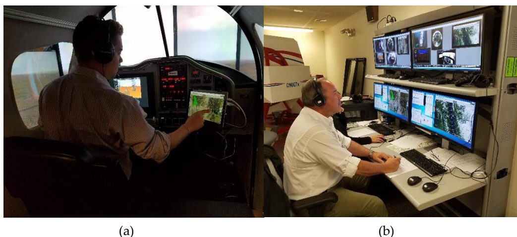
Figure 1. (a) The Flight Training Device (FTD) cockpit, configured as a Mooney aircraft; (b) air traffic control (ATC) station, with an experimenter playing the role of ATC.
