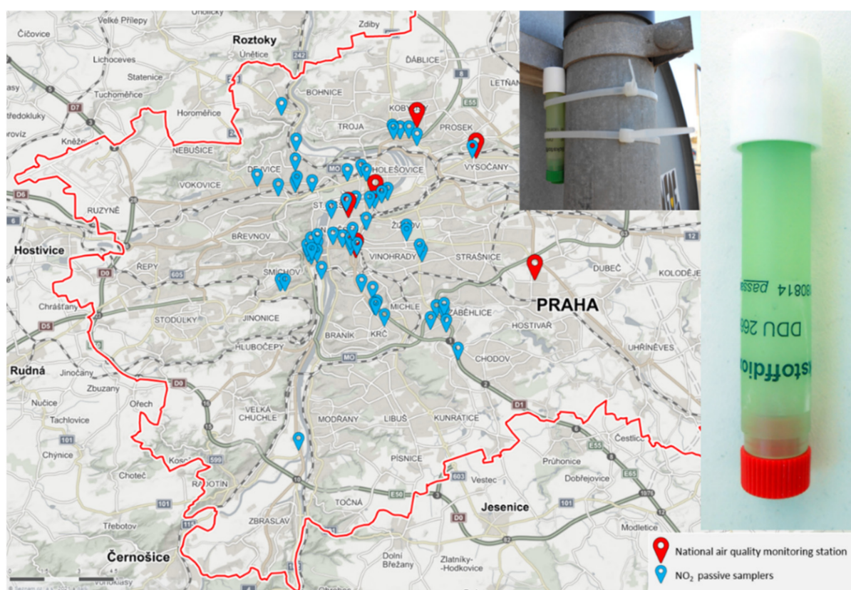
Figure 1. Locations of the passive samplers and air quality monitoring stations used for comparison in this study. Photo of a sampler is shown in the upper right corner. (Map source: www.mapy.cz (accessed on 18 May 2021), © Seznam.cz, a.s., used with permission).
