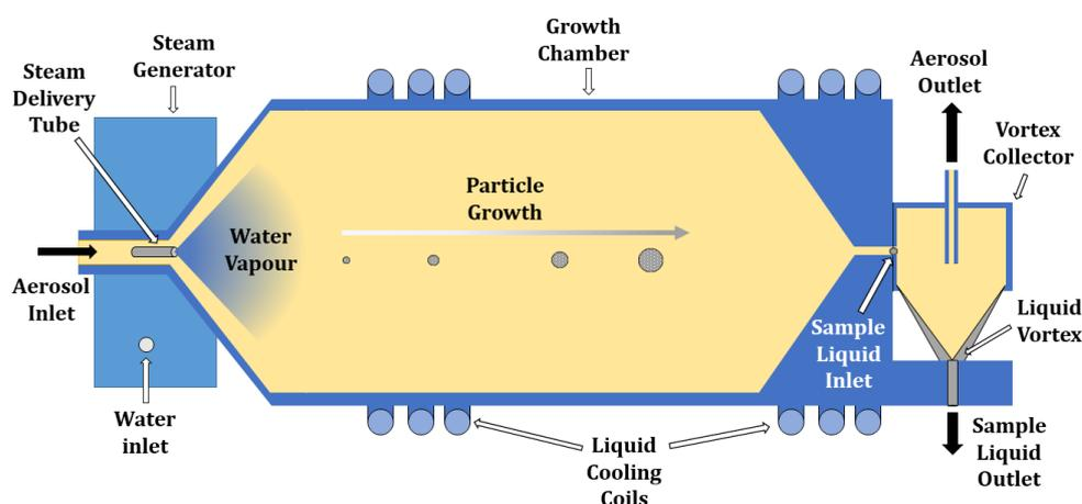
**Figure 2.** PINQ insoluble aerosol collector (IAC) diagram, highlighting major components such as the aerosol input, steam generator, growth chamber, and vortex collector. (Figure adapted from Brown et al. [42]).
