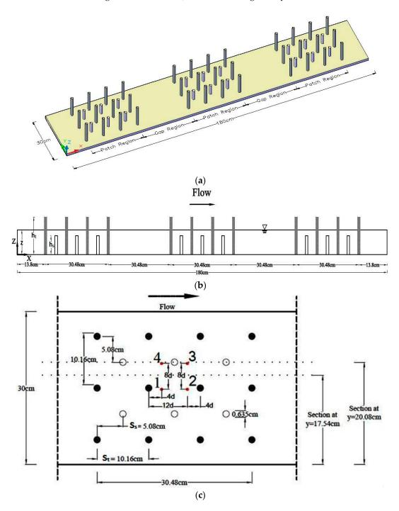
**Figure 3.** Schematic diagrams of the domain: (**a**) isometric view of the domain; (**b**) vertical section of the discontinuous patch configuration; and (**c**) top view of the last vegetation patch showing critical locations in red color (i.e., Locations 1, 2, 3, and 4).
