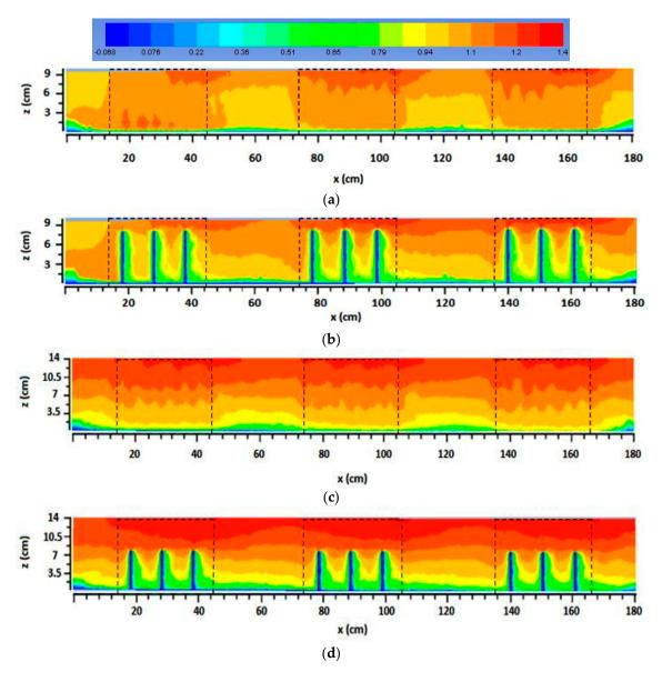
**Figure 6.** Contour diagrams of the mean velocity u/U for Case A at sections (**a**) y = 17.54 cm and (**b**) y = 20.08 cm; and for Case B at sections (**c**) y = 17.54 cm and (**d**) y = 20.08 cm. The dashed boxes represent the area occupied by the vegetation patches.
