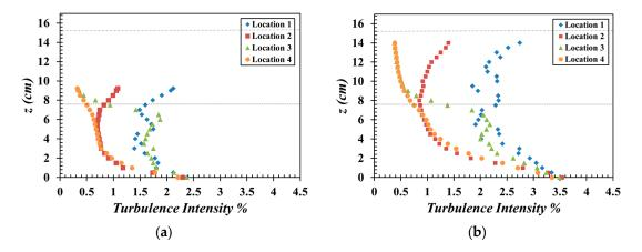
**Figure 12.** Turbulence intensity (%) profiles at critical locations (1, 2, 3, and 4) (**a**) for Case A, and (**b**) for Case B.
