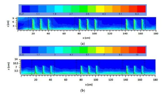
**Figure 13.** Distribution of turbulence intensity (%) at section y = 20.08 cm (**a**) for Case A, and (**b**) for Case B.
