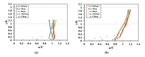
**Figure 4.** Vertical profiles of mean streamwise velocities at various locations of section y = 17.54 cm (a) for Case A, and (b) for Case B. For the meaning of *x* and *y*, see the caption of Figure 3.
