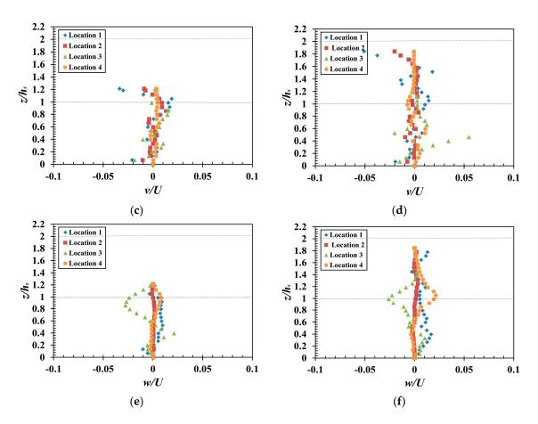
**Figure 5.** Vertical profiles of mean streamwise (*u*), transverse (*v*), and vertical (*w*) velocities at critical locations (1, 2, 3, and 4) for Case A (**a**, **c**, **e**) and for Case B (**b**, **d**, **f**). For the definition of the four critical locations, see Figure 3c.
