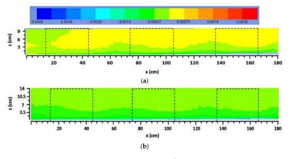
**Figure 10.** Contour diagrams of Reynolds stresses  $(u'w'/U^2)$  (a) for Case A, and (b) for Case B.
