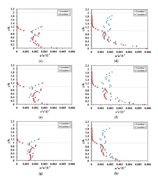
**Figure 8.** Simulated profiles of Reynolds stresses and normal stresses at critical typical locations (1 and 3) for Case A (**a**, **c**, **e**, **g**) and for Case B (**b**, **d**, **f**, **h**). The lower and upper dotted lines represent the top of vegetation layers 1 and 2, respectively.
