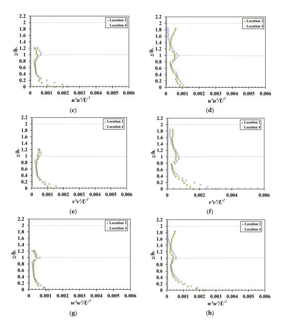
**Figure 9.** Simulated profiles of Reynolds stresses and normal stresses at typical locations (2 and 4) for Case A (**a**, **c**, **e**, **g**) and for Case B (**b**, **d**, **f**, **h**). The lower and upper dotted lines represent the top of vegetation layers 1 and 2, respectively.
