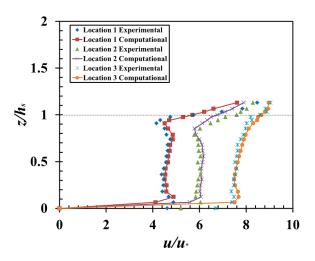
**Figure 2.** Comparison of simulated velocity profiles with the experimental data of Liu et al. [27]. The dotted line shows the top of submerged vegetation.
