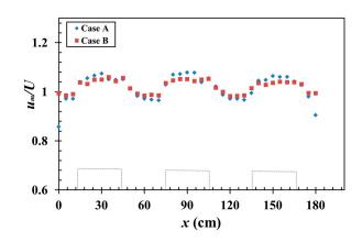
**Figure 7.** Fluctuations of depth-averaged mean velocity along the length for both Case A and Case B. The dashed boxes denote the vegetation patches.
