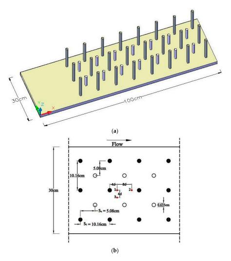
**Figure 1.** Experimental model geometry of Liu et al. [27] in (**a**) isometric view, and (**b**) close top view showing specific locations (i.e., 1, 2, 3) in red color.
