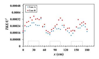
**Figure 11.** Deviations of depth-averaged turbulent kinetic energy along length for both Case A and Case B. The dashed boxes denote the vegetation patches.
