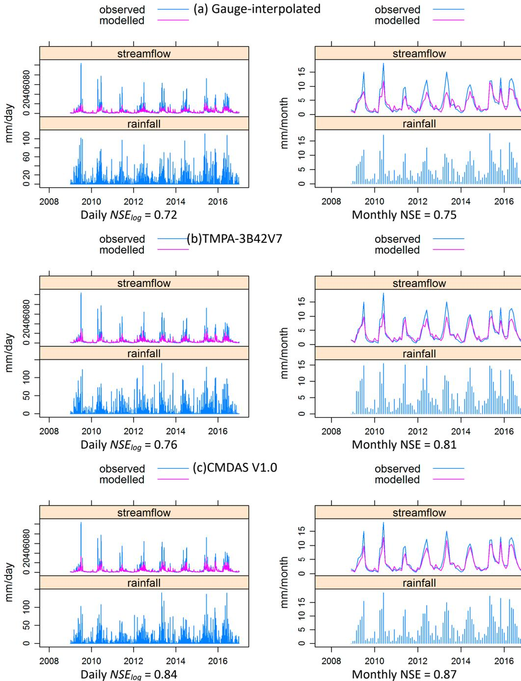
**Figure S3.** Observed and Sacramento-model-simulated daily and monthly runoffs for (a) Gauge-interpolated, (b) TMPA-3B42V7 and (c) CMDAS rainfall datasets (for the Sacramento model calibrated using  $NSE_{log}$  as the objective function).
