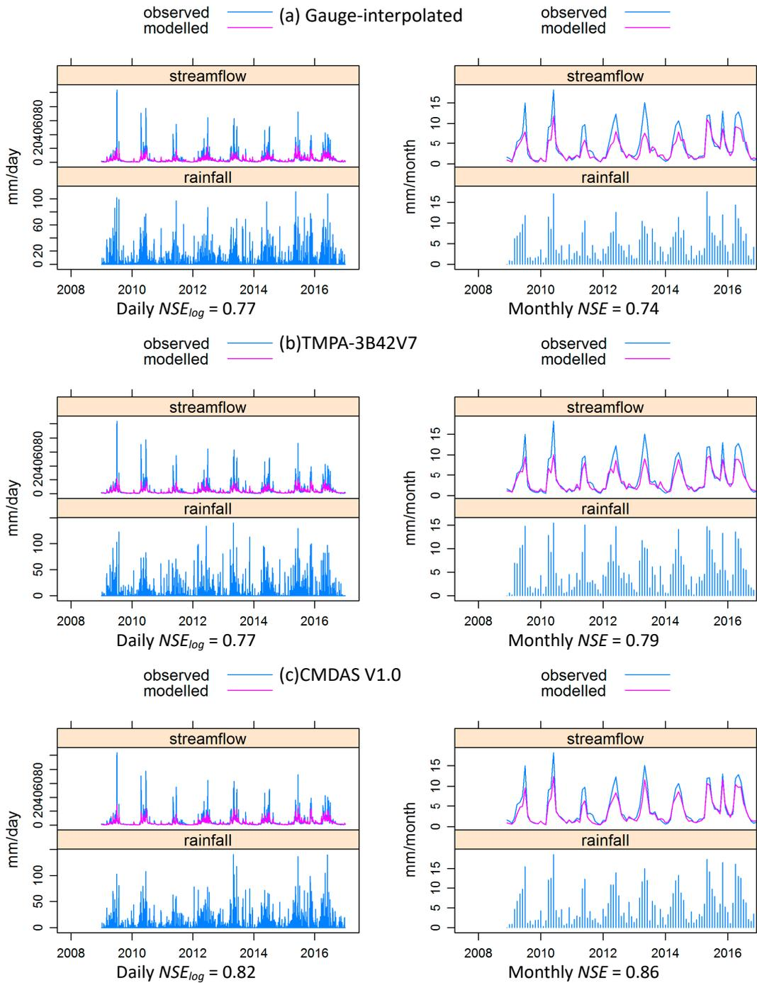
**Figure S2.** Observed and IHACRES-model-simulated daily and monthly runoffs for (a) Gauge-interpolated, (b) TMPA-3B42V7 and (c) CMDAS rainfall datasets (for the IHACRES model calibrated using  $NSE_{log}$  as the objective function).
