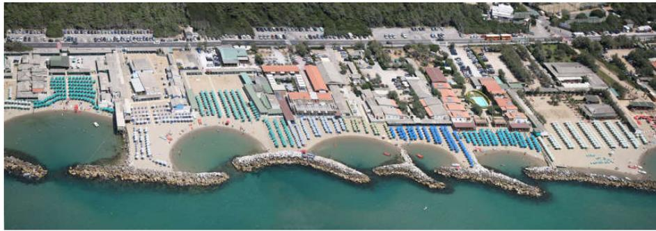
**Figure 15.** Between Marina di Pisa and Tirrenia: coastal armoring following emergency, un-coordinated interventions (Photo Provincia di Livorno).
