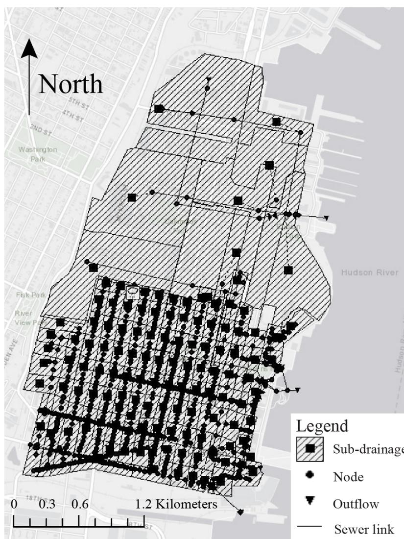
**Figure 4.** Sewer network of the City of Hoboken as implemented in SWMM [53].
