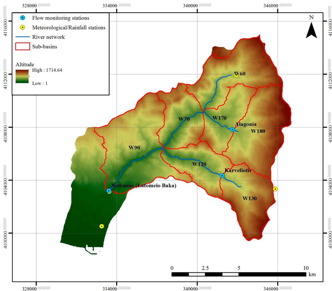
**Figure 4.** Digital map of Nedontas River Basin, also showing monitoring stations (meteorological and hydrometric) and the main modelling components (junctions, sub-basins, river segments).
