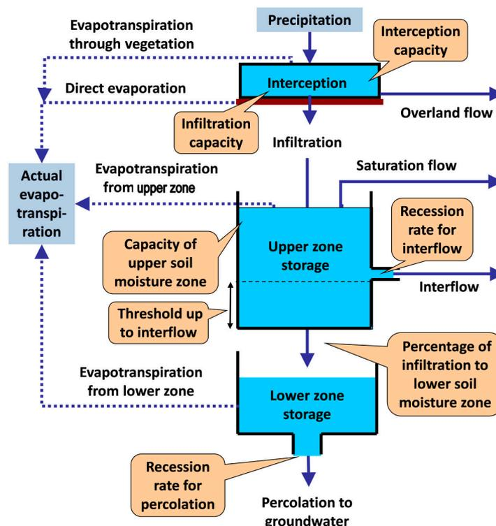
**Figure A1.** Representation of modelling components and associated fluxes within basin partitions. Meteorological inputs (Precipitation (PET)) vary across sub-basins, while model parameters, shown in callouts, vary across HRUs.
