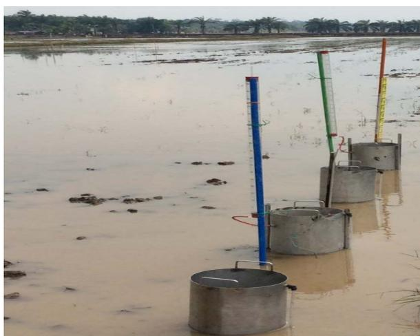
**Figure 3.** Monitoring daily percolation rate using field lysimeters in the experimental plot.
