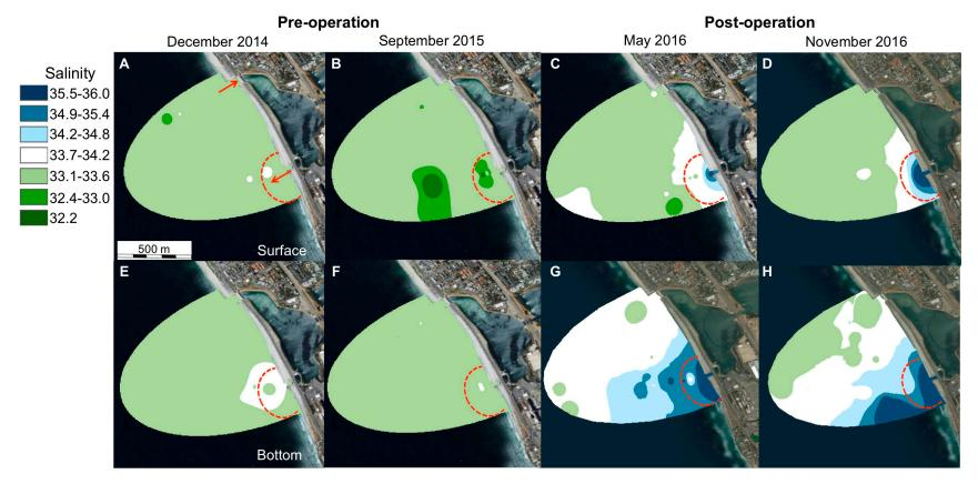
**Figure 2.** GIS-mapped salinity measurements for surface (**upper row**) and bottom water (**lower row**) for pre-operation (**A**,**B**,**E**,**F**) and post-operation (**C**,**D**,**G**,**H**). Arrows in (**A**) indicate the outfall location and lagoon intake area. The red semi-circle represents the 200 m distance set by California Ocean Plan (2015 Amendment to the Water Quality Control Plan).
