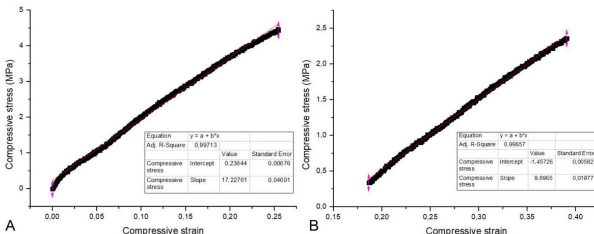
**Figure 6.** Estimation of modulus of elasticity from (A) seabreams without any skeletal deformity and (B) seabreams with scoliosis.
