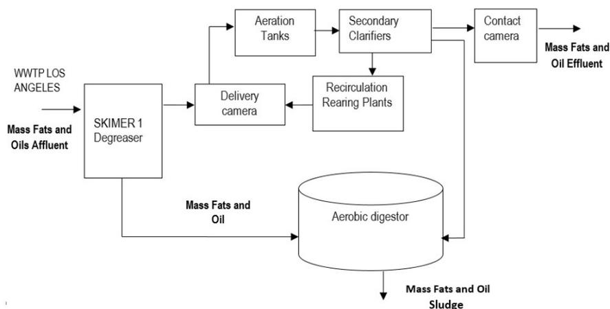
**Figure 4.** General flow diagram of the Los Angeles WWTP.
