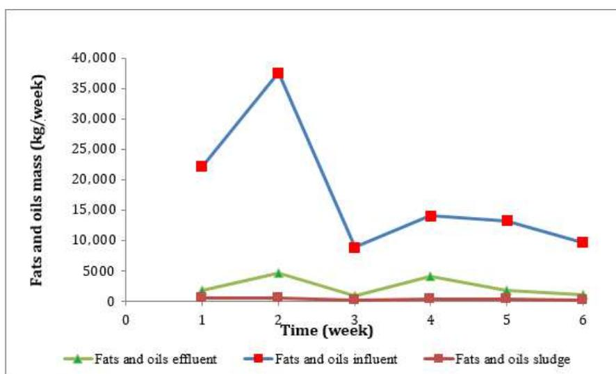
**Figure 6.** Weekly changes in mass of fats and oils in real scale wastewater treatment plant.
